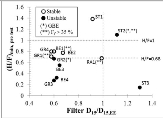
**Figure 5:** The stability index pre-test (initial) gradation versus the excessive erosion boundary (EE).
