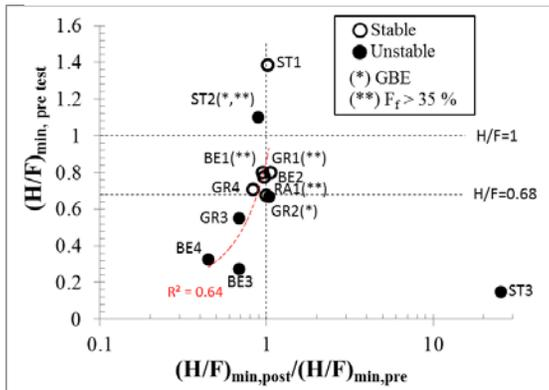
**Figure 7:** The stability index pre-test (initial) gradation versus the stability index ratio of the post-test gradation (layer 4). The exponential trend line is established for samples with  $F_f < 35\%$  (ST3 not considered).
