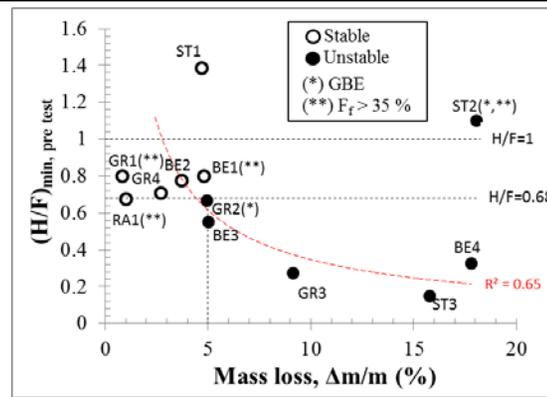
**Figure 6:** The stability index pre-test (initial) gradation versus the mass loss in the downward flow permeameter test. The power trend line is established for samples with  $F_f < 35\%$ .
