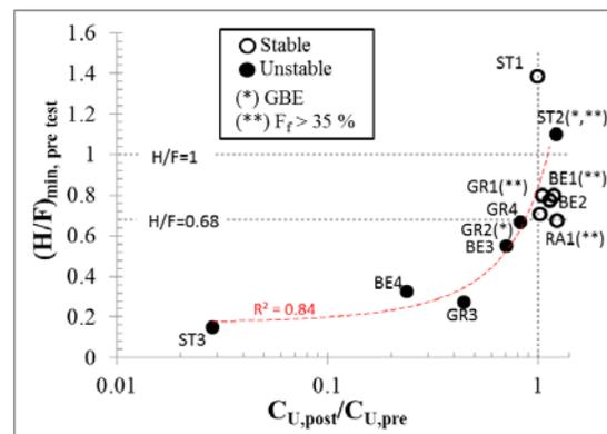
**Figure 8:** The stability index pre-test (initial) gradation versus the coefficient of uniformity ratio of the post-test gradation (layer 4). The exponential trend line is established for samples with  $F_f < 35\%$ .
