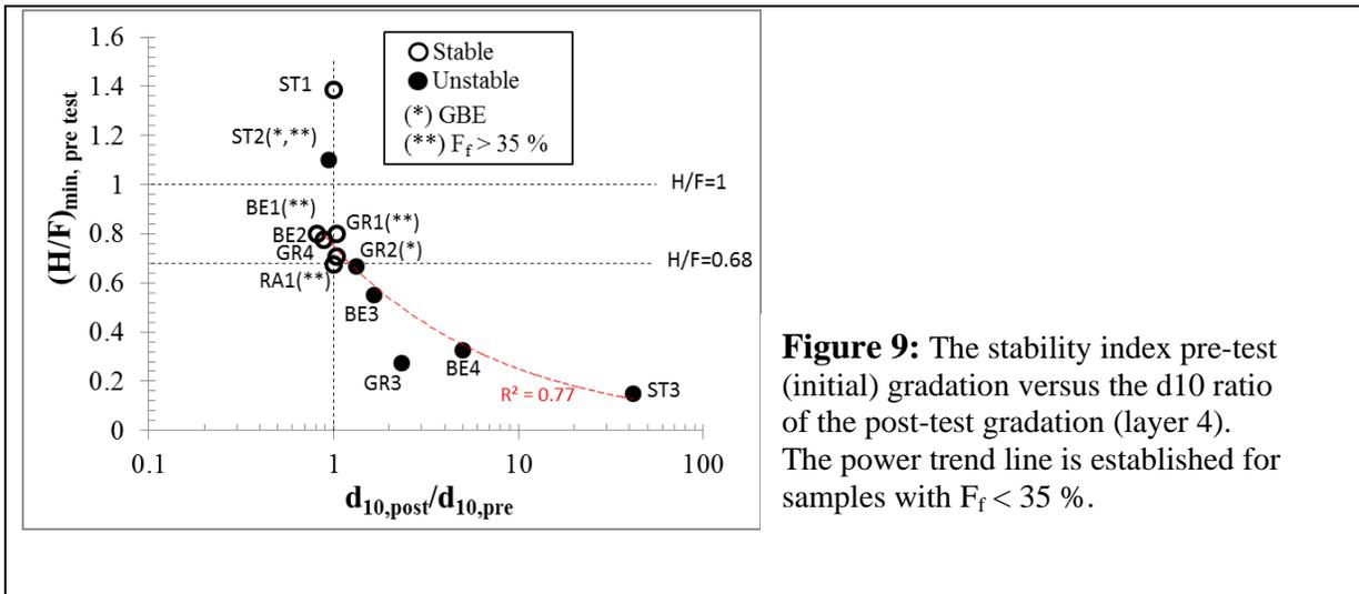
**Figure 9:** The stability index pre-test (initial) gradation versus the d10 ratio of the post-test gradation (layer 4). The power trend line is established for samples with  $F_f < 35\%$ .
